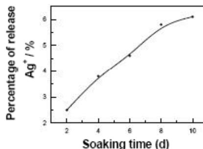
Figure 3: The percentage of release Ag<sup>+</sup> in 4<sup>#</sup> sample soaking in deionized water for different time
