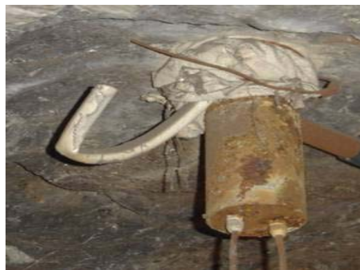
Figure 10 : Field test scene of multiple point displacement meter
