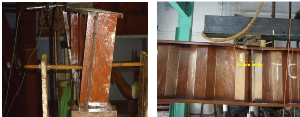
Fig. 4 (a): Lateral torsional buckling (b) Bearing failure
