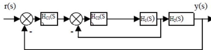
**Figure 2 : The main steam temperature control system controlled by cascade**
