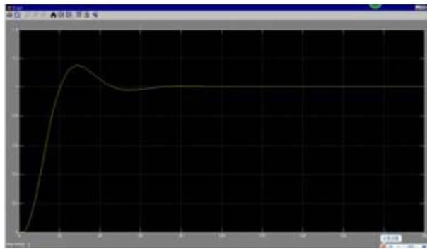
Figure 4 : Z -N setting system response curve
