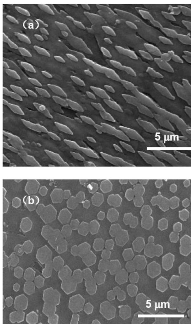
Figure 1: (a) The typical SEM pictures of pearls in the control group. Many rhombus or spindly crystal slices are uniformly located on the surface with an angle of 30° to horizontal. (b) Many regular hexagonal blocks are seen on the top surface, without any overlap or aggregation. Each block has a perfect regular hexagonal structure
