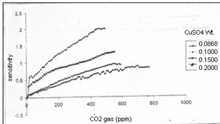
**Fig. 1: Sensitivity variation with concentration of CO<sub>2</sub> at room temperature (301 K)**
