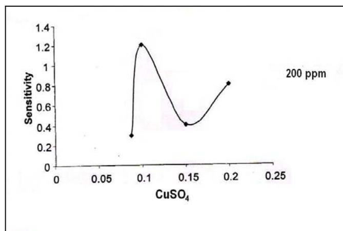
**Fig. 3: Variation of sensitivity against  $\text{CuSO}_4 \cdot 5\text{H}_2\text{O}$  concentration**
