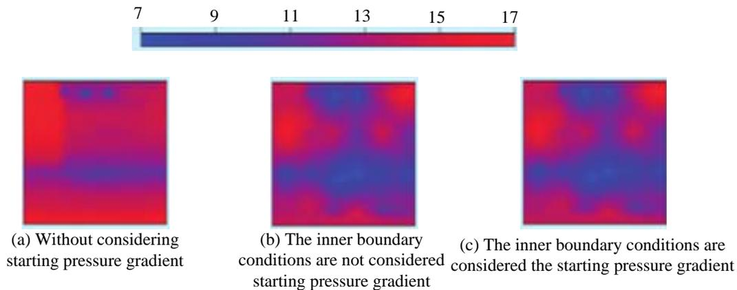
Figure 5 : Pressure distributions to consider different factors
