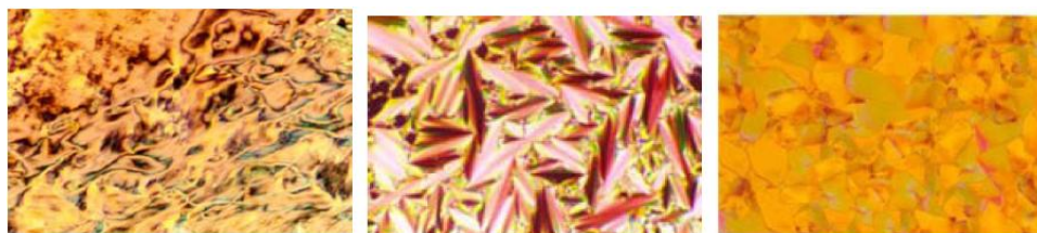
Figure 2: Microphotographs showing (a) Schlieren texture of lyotropic nematic phase (180X); (b) Focal conic fan shaped texture of SmA phase (180X); (c) Broken banded focal conic fan texture of chiral Sm G phase (180X)
