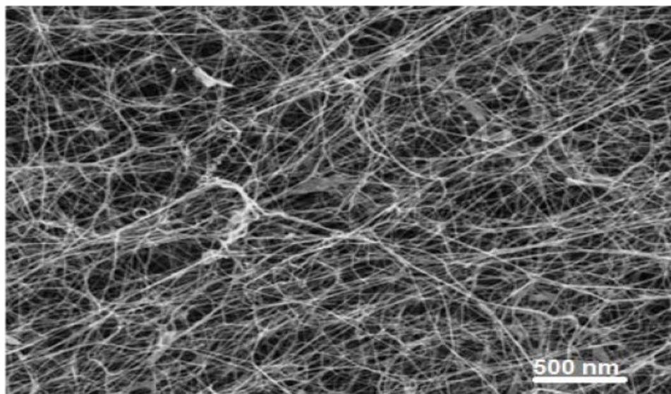
Figure 3 : SEM-image of bacterial nanocellulose
