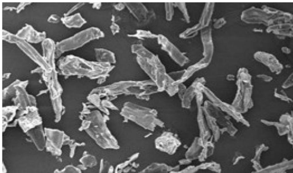
Figure 4 : Micro-photograph of microcrystalline cellulose (magnification 300 x)
