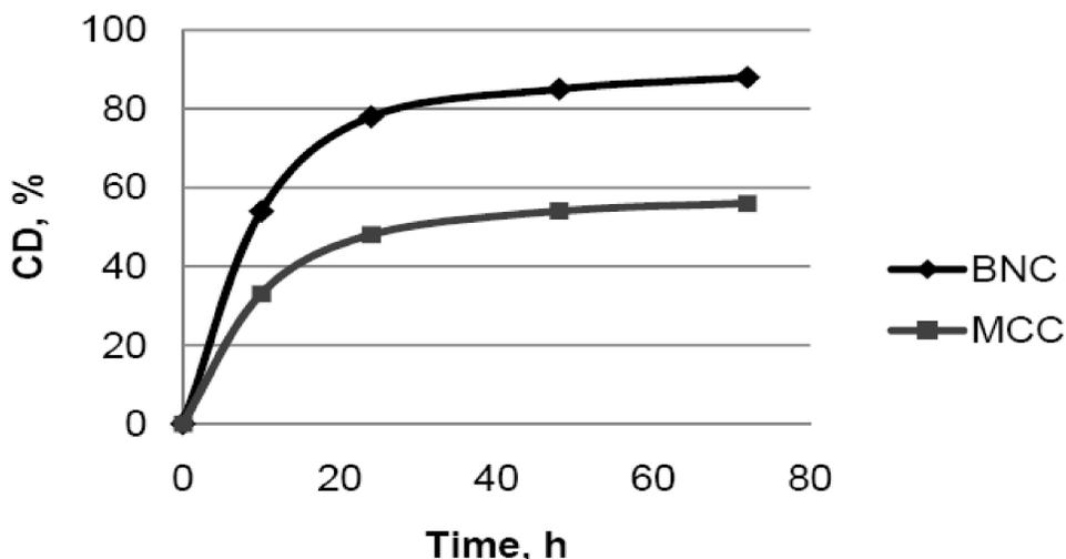
Figure 1 : Kinetic curves of enzymatic hydrolysis of never-dried cellulose samples
