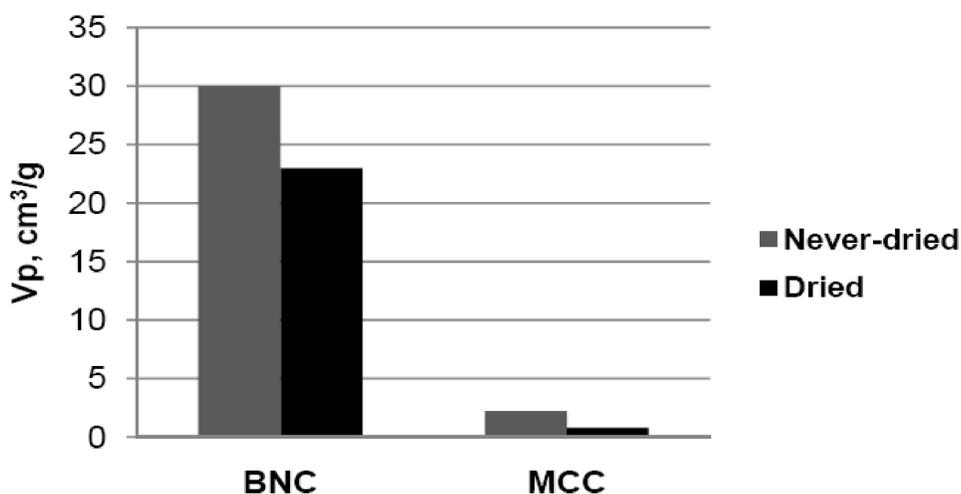
Figure 5 : Porosity of the never-dried and dry cellulose samples
