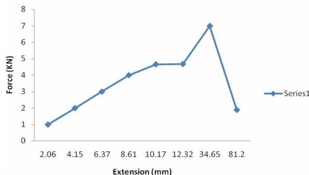
Figure 4 : Tensile property of VHDPE plastic showing deformation force versus extension
