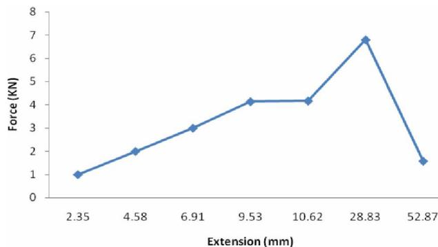
Figure 6 : Tensile property of VRHDPE plastic showing deformation force versus extension
