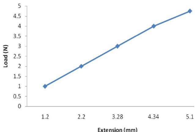
Figure 2 : Flexural property of TRHDPE plastic showing the Loading versus bending extension
