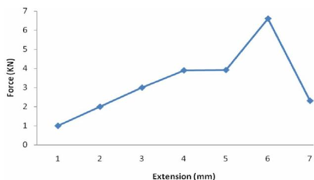
Figure 5 : Tensile property of TRHDPE plastic showing deformation force versus extension
