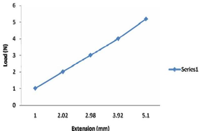
Figure 1 : Flexural property of VHDPE plastic showing the Loading versus bending extension
