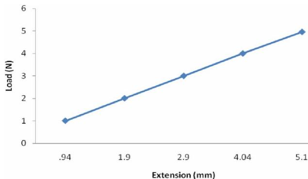
Figure 3 : Flexural property of VRHDPE plastic showing the loading versus bending extension
