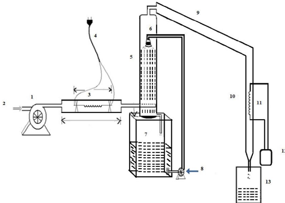
1-blower, 2-air inlet flow, 3- air heater, 4-electric plugin, 5-humidifier, 6-water sprinkle, 7-raw water tank, 8-pump, 9-air carrier, 10 -dehumidifier, 11-refrigerator coil surface, 12-compressor, 13-treated water.
