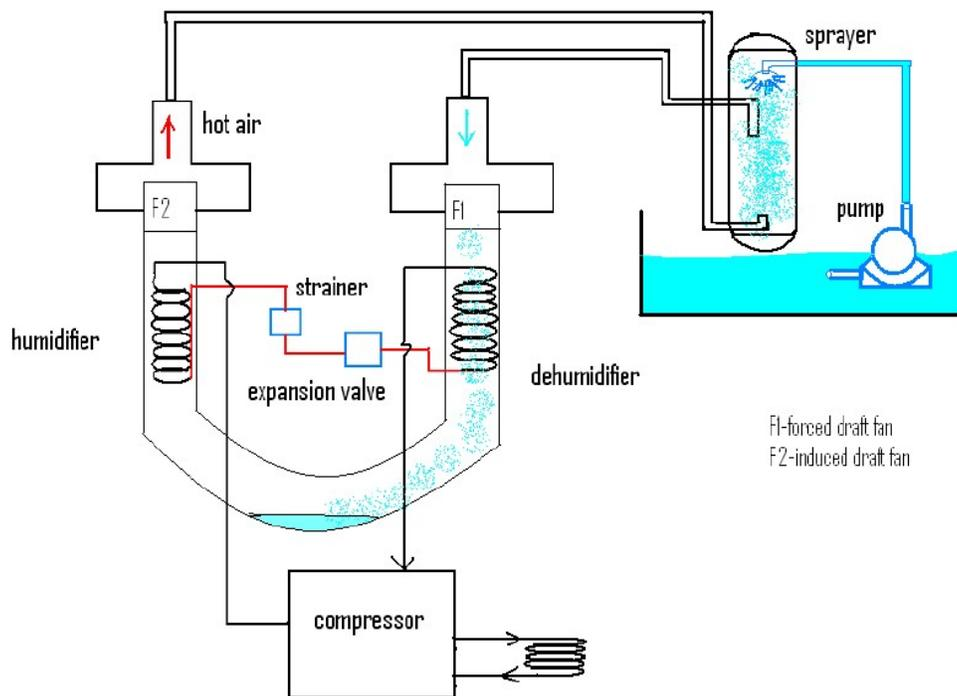
Figure 1 : Diagram of closed loop system
