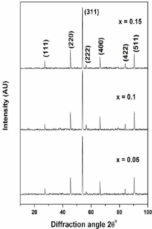
Figure 1 : X-ray diffraction (XRD) patterns of  $\text{Co}_{0.7-x}\text{Ni}_x\text{Mn}_{0.3}\text{Fe}_2\text{O}_4$  system
