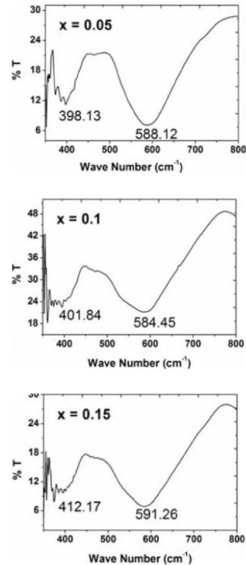
Figure 2 : The IR absorption bands of  $\text{Co}_{0.7-x}\text{Ni}_x\text{Mn}_{0.3}\text{Fe}_2\text{O}_4$  system
