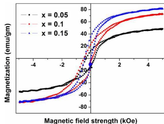
Figure 4 : B-H loops of  $\text{Co}_{0.7-x}\text{Ni}_x\text{Mn}_{0.3}\text{Fe}_2\text{O}_4$  system
