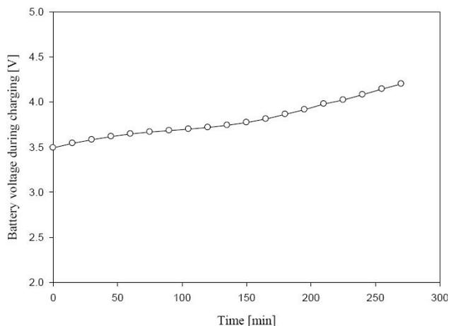
**Figure 8 : Battery voltage during charging versus time when charged at a rate of 9 A**
