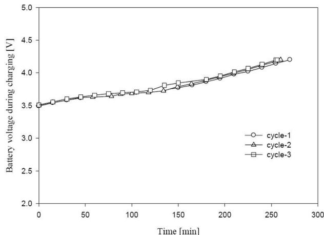
**Figure 9 : Comparison of charging voltage during three different cycles all at a same rate of 9 A**
