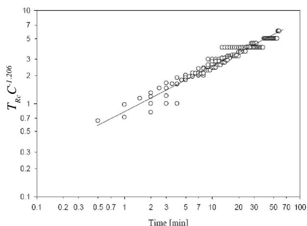
**Figure 11 : Correlation plot for anode temperature rise according to eqn.2.**
