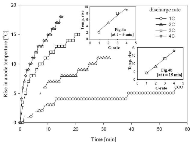
**Figure 4 :** Variation of rise in anode temperature versus time at different C-rates
