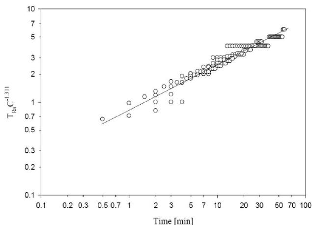
**Figure 10 : Correlation plot for anode temperature rise according to eqn.1.**
