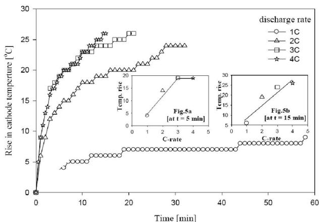
**Figure 5 :** Variation of rise in cathode temperature versus time at different C-rates
