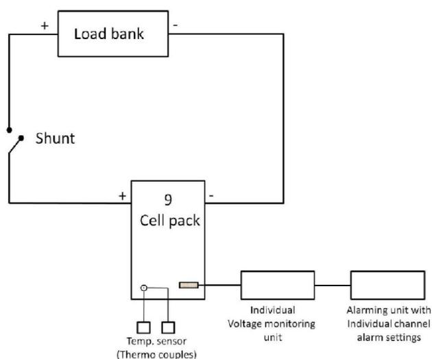
**Figure 1 : Electric circuit for carrying out discharge studies**
