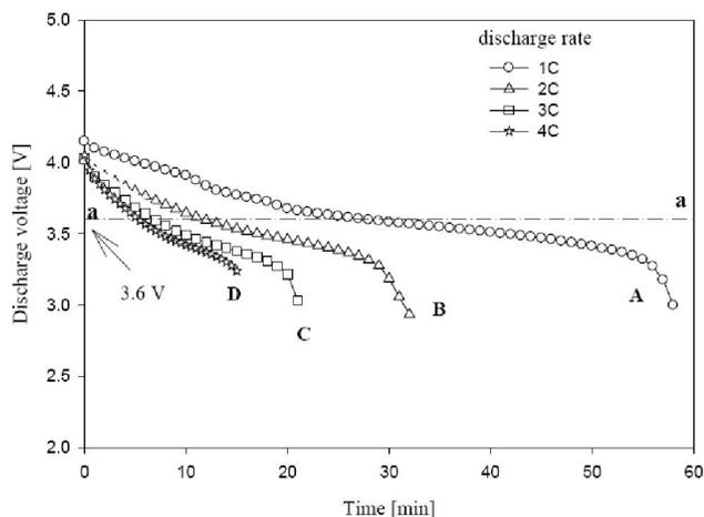
Figure 3 : Discharge voltage versus time at different C-rates
