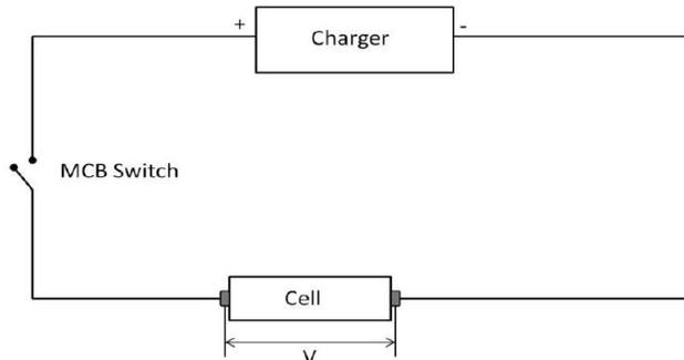
**Figure 2 : Electric circuit for charging battery**
