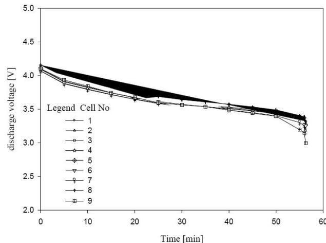
**Figure 6 :** Discharge voltage of all nine cells in a 9-cell pack at 1C rate
