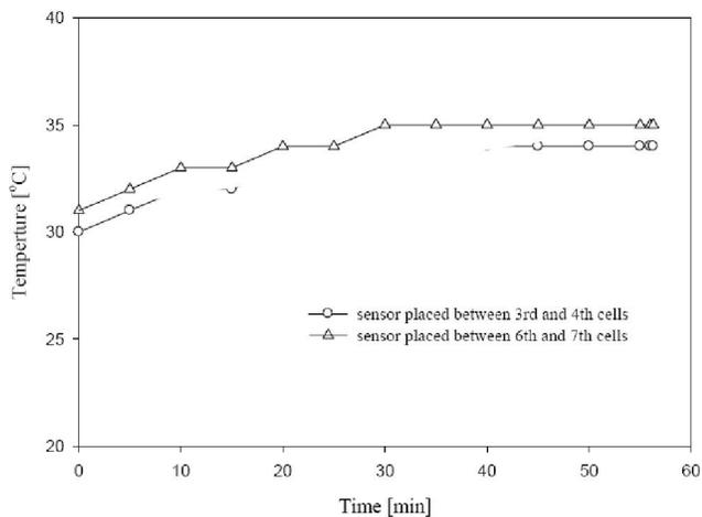
**Figure 7 : Variation of temperature of 9-cell pack at select points versus time when discharging at 1C rate**
