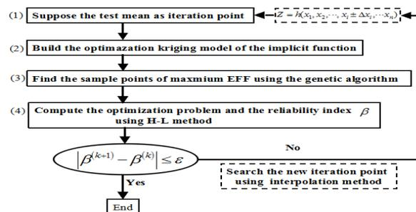
FIGURE 2 Computation procedure of the reliability index
