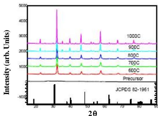
Figure 3: The powder X-ray diffraction pattern of  $\text{La}_{0.6}\text{Sr}_{0.2}\text{Ca}_{0.2}\text{Co}_{0.2}\text{Fe}_{0.8}\text{O}_3$  (LSCCF) calcinated at temperatures of 600, 700, 800, 900 and 1000°C
