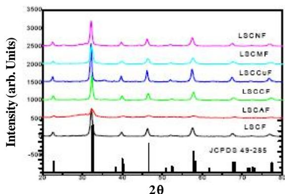
Figure 2: The powder X-ray diffraction pattern at temperature 600°C calcined for 4hrs  $\text{La}_{0.6}\text{Sr}_{0.2}\text{Ca}_{0.2}\text{FeO}_3$  (LSCF) and  $\text{La}_{0.6}\text{Sr}_{0.2}\text{Ca}_{0.2}\text{M}_x\text{Fe}_{0.8}\text{O}_3$  (M=Al, Cu, Co, Mn, Ni)(LSCMF)
