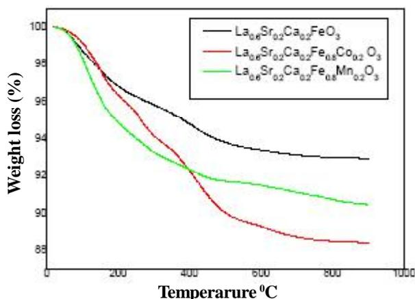
Figure 1: The TGA curve of the as synthesized powders recorded in air at a heating rate of 10°C
