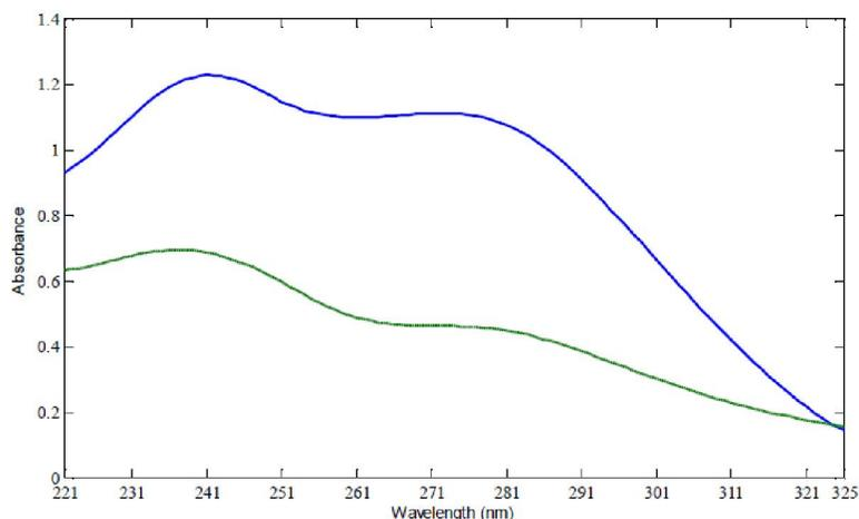
Figure 2 : Zero order spectra of (30µg / mL) Ceftriaxone ( ) and (30µg/ mL) degradate (.....).
