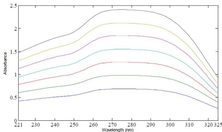
Figure 3 : Ratio spectra of ceftriaxone (6-24µg/mL) using (24µg/mL) of degradate as a divisor
