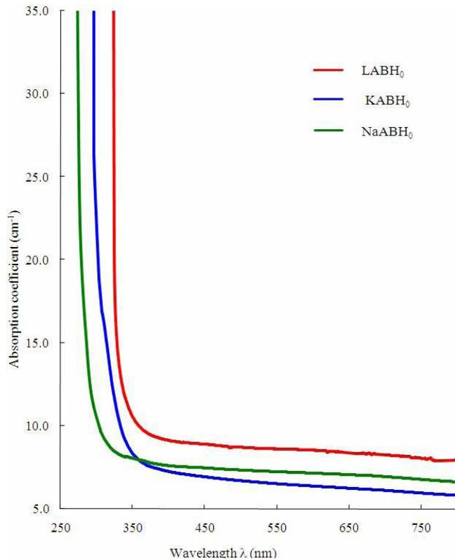
Figure 1: Optical absorption spectra of LiF/NaF/KF-Al<sub>2</sub>O<sub>3</sub>-B<sub>2</sub>O<sub>3</sub> glass recorded at room temperature
