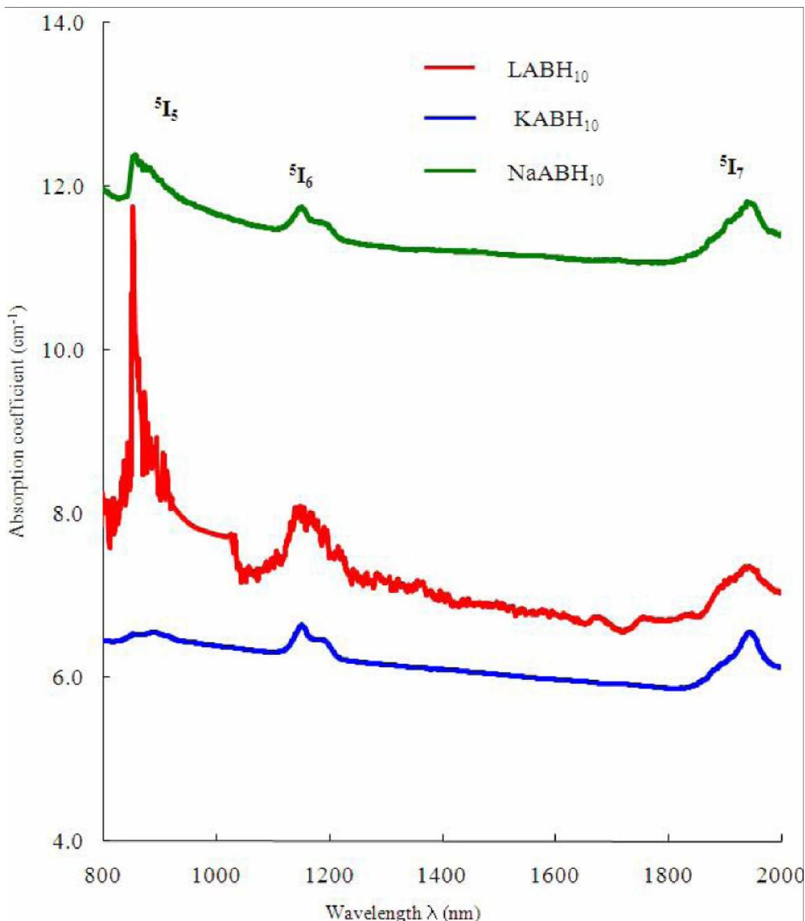
Figure 4 : Optical absorption spectra of LiF/NaF/KF-Al<sub>2</sub>O<sub>3</sub>-B<sub>2</sub>O<sub>3</sub> glass doped with 1.0 mol% of Ho<sub>2</sub>O<sub>3</sub> recorded at room temperature (NIR region)
