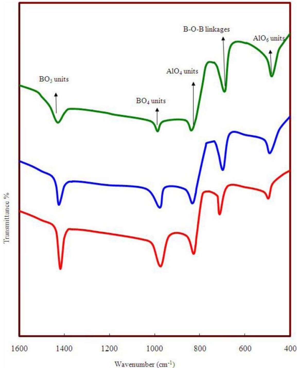
Figure 5 : FT-IR spectra of LiF/NaF/KF- $\text{Al}_2\text{O}_3$ - $\text{B}_2\text{O}_3$  glasses
