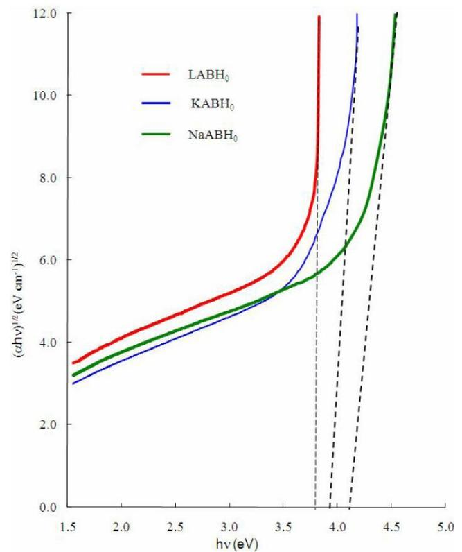
Figure 2: Tau'c plots for evaluating the optical band gap of LiF/NaF/KF-Al<sub>2</sub>O<sub>3</sub>-B<sub>2</sub>O<sub>3</sub> glass
