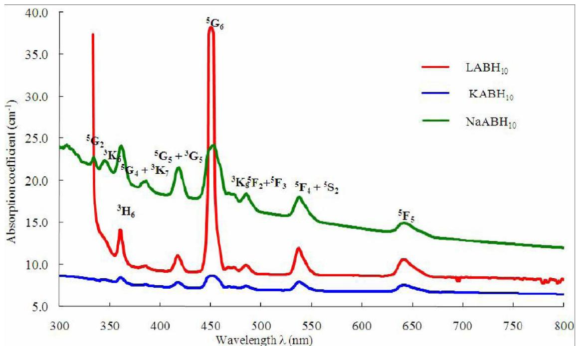
Figure 3: Optical absorption spectra of LiF/NaF/KF-Al<sub>2</sub>O<sub>3</sub>-B<sub>2</sub>O<sub>3</sub> glass doped with 1.0 mol% of Ho<sub>2</sub>O<sub>3</sub> recorded at room temperature
