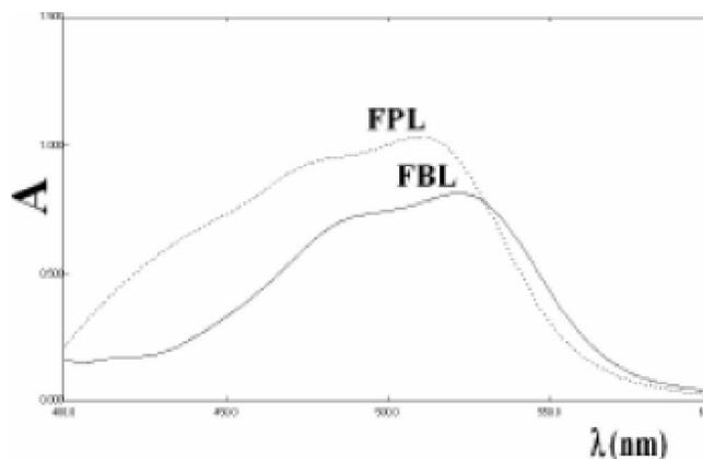
Figure 1 : Absorption spectra of FPL and FBL complexes in presence of 4.0 ppm Mf.
