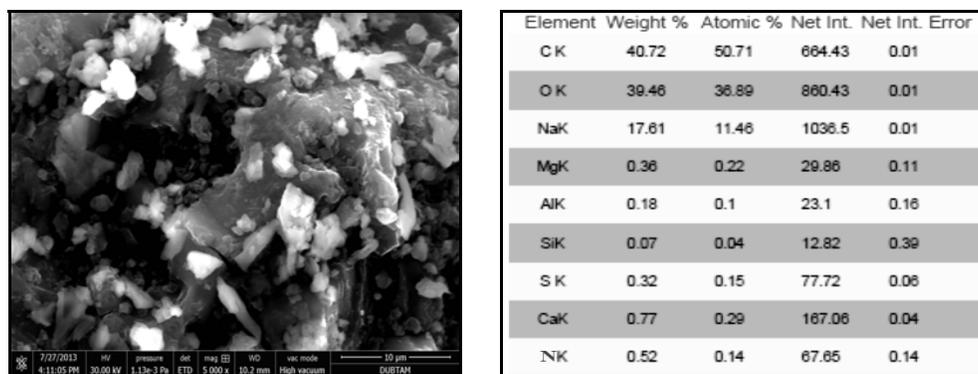
Fig. 1: The SEM image and EDAX results of sodium humate
