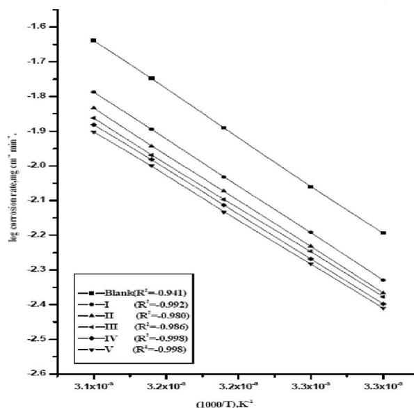
**Figure 4 :** log corrosion rate vs.  $1/T$  curves for 304 SS dissolution in absence and presence of  $9 \times 10^{-6}$  M of inhibitors
