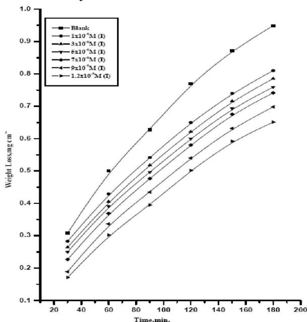
**Figure 1 :** Weight loss - time curves for the dissolution of 304 SS in the absence and presence of different concentrations of compound (I) at 30°C
