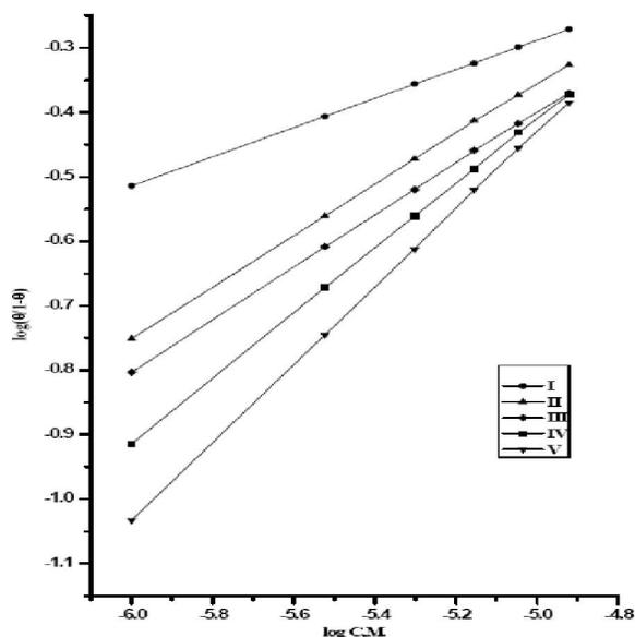
**Figure 3 :** Curve fitting of corrosion data for 304 SS in 3M HCl in the presence of different concentrations of Thiophene derivatives to kinetic model
