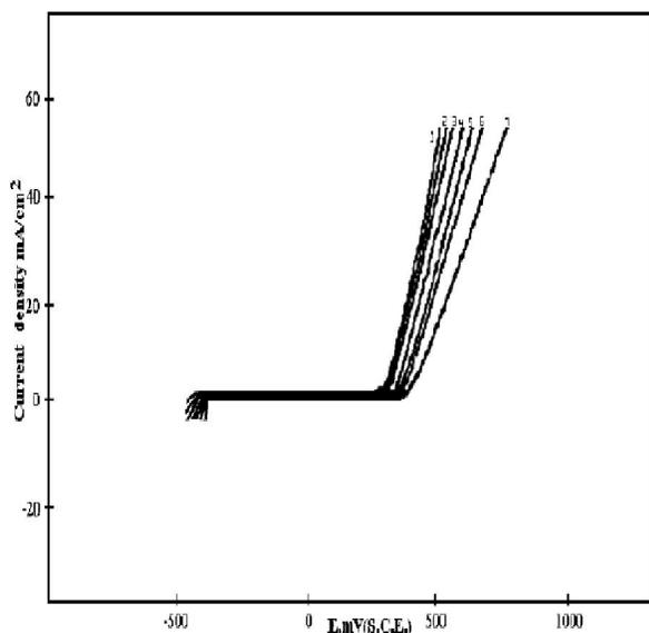
**Figure 7 : Potentiodynamic anodic Polarization curves of 304 SS in 3.5 % NaCl containing different concentrations of compound (I)**
