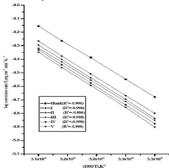
Figure 5 : log corrosion rate/T vs.1/T curves for 304 SS dissolution in the absence and presence of  $9 \times 10^{-6}$  M of inhibitors
