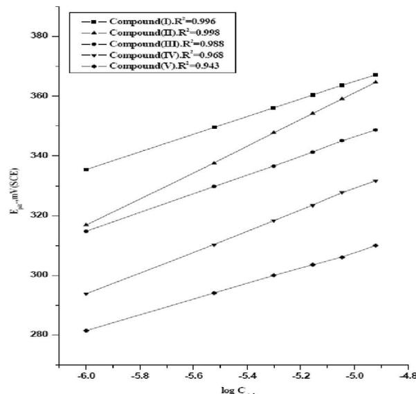
**Figure 8 : The relationship between pitting potential of 304 SS and logarithm the concentration of the additives in presence of 3.5 % NaCl**
