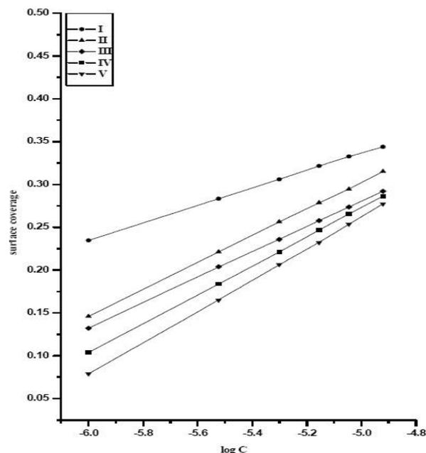
**Figure 2 :**  $\theta$ -log C curves for 304 SS in 3M HCl in the presence of all inhibitors from weight loss measurements at 30°C
