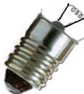
Figure 3 : A miniature IR source constructed from a 2.5V lamp by removing its glass envelope.
