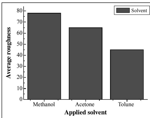
**Fig. 6: The calculated AFM-roughness as a function of applied solvent**
