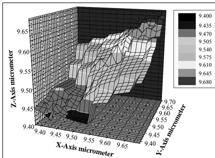
**Fig. 4a:** 3D-AFM-mapping surface of highly pure metformin crystallized from methanol
