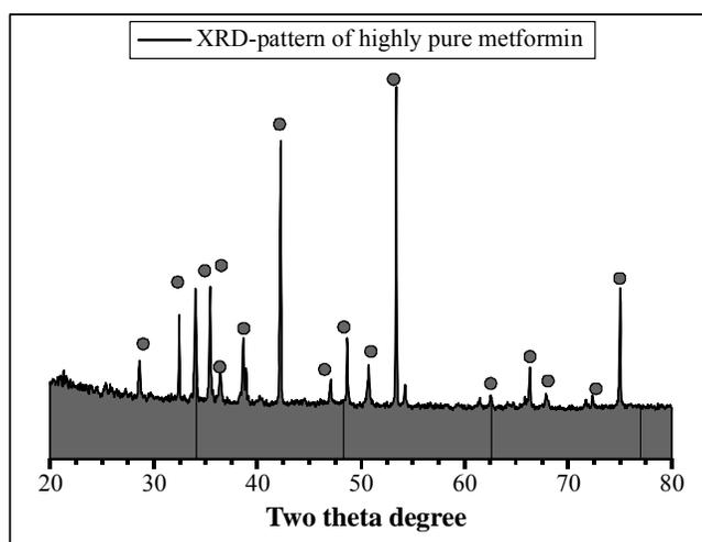
**Fig. 2: XRD pattern recorded for highly pure metformin extracted from methanol**
