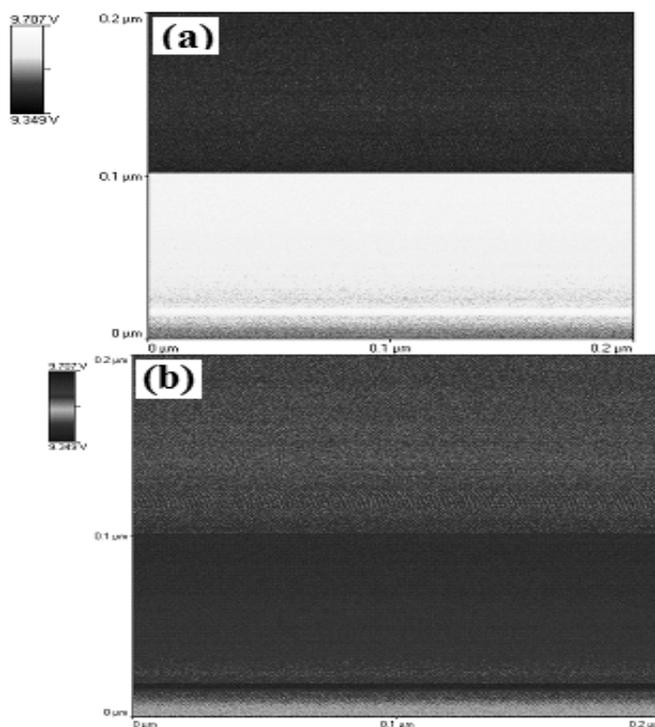
**Fig. 5: AFM-micrographs recorded for metformin extracted from (a) toluene and (b) acetone, respectively**
