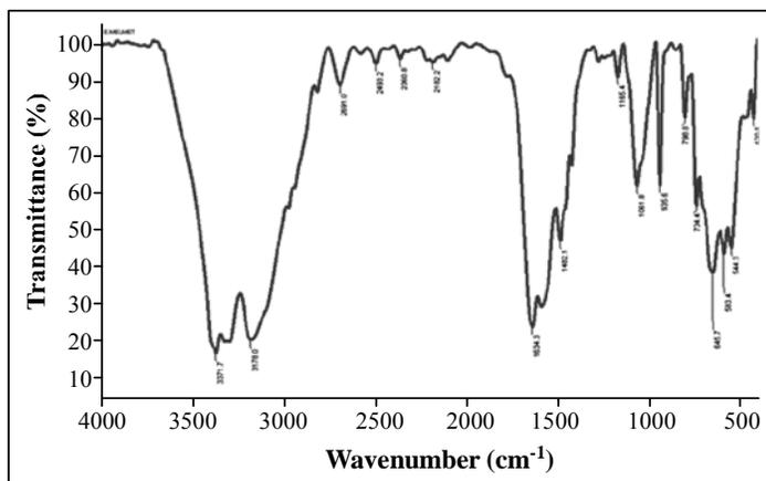
**Fig. 3:** FT-IR spectra recorded for pure metformin
