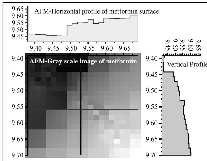
**Fig. 4b: AFM-Horizontal/Vertical profiles of metformin surface extracted from methanol**
