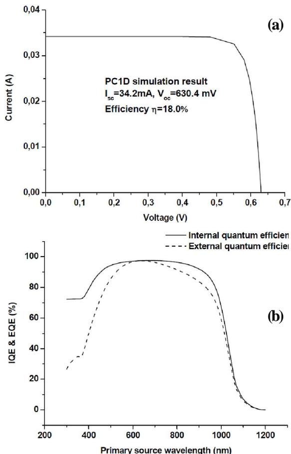
Figure 2 : PC1D 5.9 simulation results for  $\text{SiN}_x/\text{Si}(n^+)/\text{Si}(p)/\text{Si}(p^+)$  : (a)  $I(V)$ , (b) quantum efficiency.
