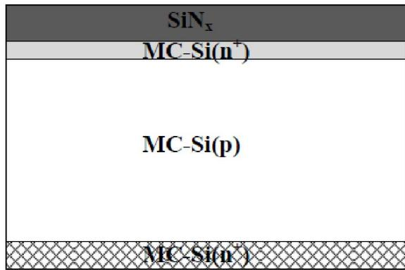
Figure 1 :  $\text{SiN}_x/\text{Si}(n^+)/\text{Si}(p)/\text{Si}(p^+)$  multi-crystalline silicon based solar cell proposed to simulation.
