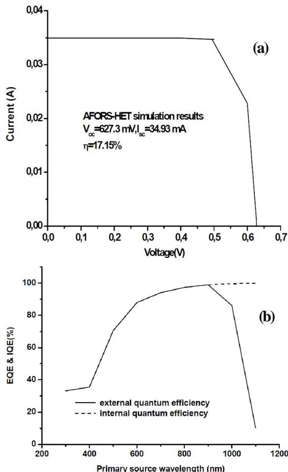
**Figure 4 :** AFORS-HET simulation results for  $\text{SiN}_x/\text{Si}(n^+)/\text{Si}(p)/\text{Si}(p^+)$  : (a)  $I(V)$ , (b) quantum efficiency.
