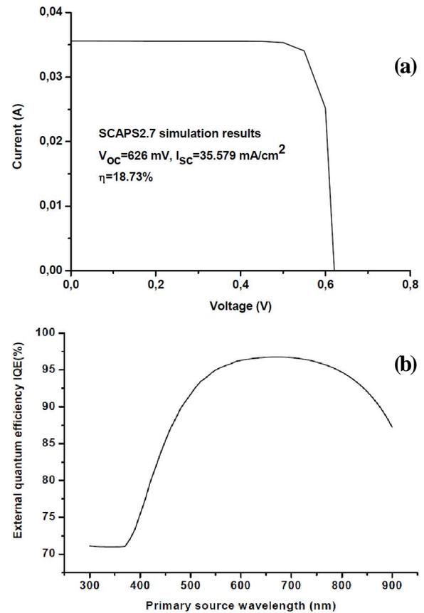
Figure 3 : SCAPS 2.7 simulation results for  $\text{SiN}_x/\text{Si}(n^+)/\text{Si}(p)/\text{Si}(p^+)$  : (a)  $I(V)$ , (b) quantum efficiency.
