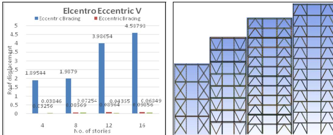
**Fig. 2: Comparison in roof displacement of conventional steel braced, SMA braced and the frames with composite arrangement subjected to EI Centro ground motion & Elevation of structures with different bracing patterns**
