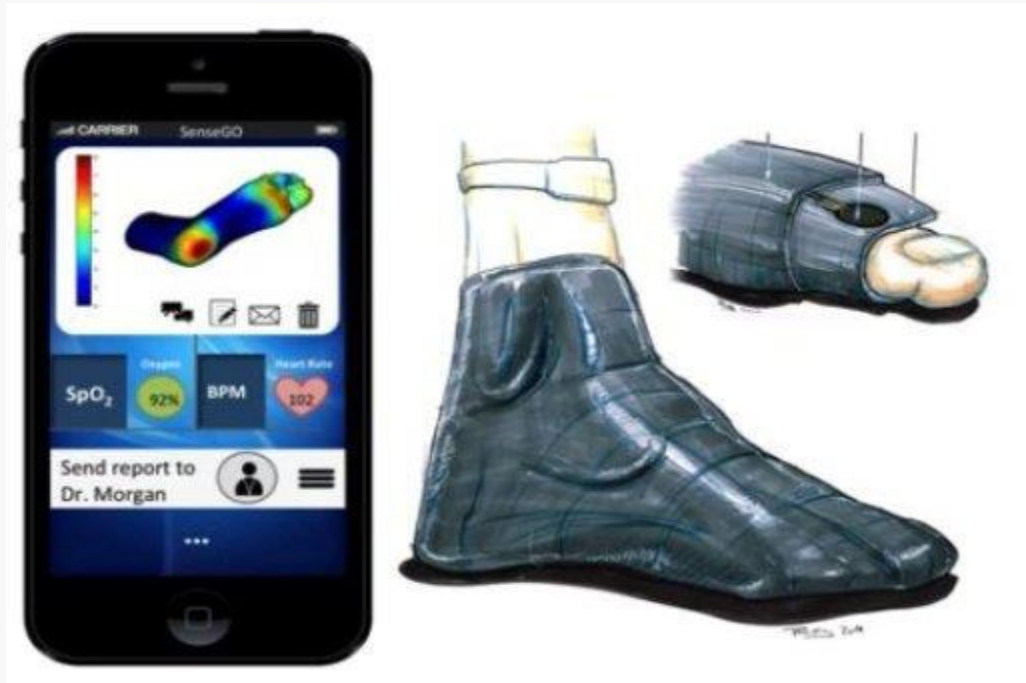
FIG. 5. Pressure-sensing socks are paired with smartphones (Reference: The Hebrew University of Jerusalem).
