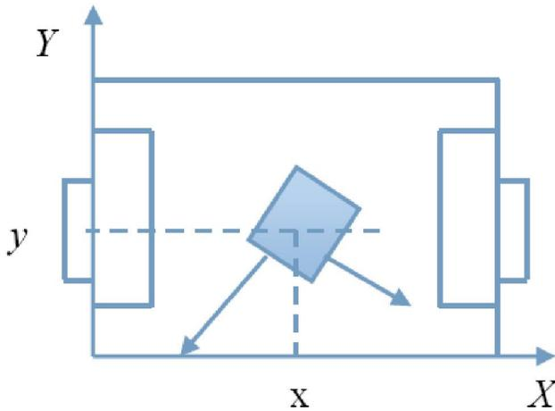
**Figure 1 : Schematic description of the position and posture of the robot**
