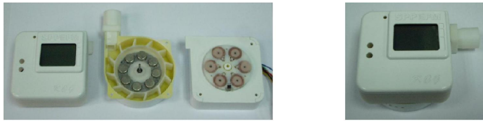
(a) LCD Panel, rotor and stator (b)The assembled equipment
