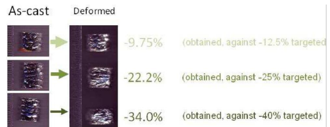
Figure 2 : The three samples destined to compression (initial and final states).
