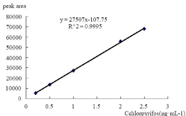
Figure 2 : The standard curve of chlorpyrifos
