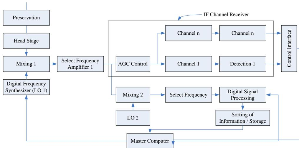
Figure 4 : Composition diagram of composite receiver
