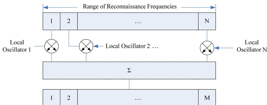
**Figure 2 : Schematic diagram of folded-frequencies information channelized receiver**
