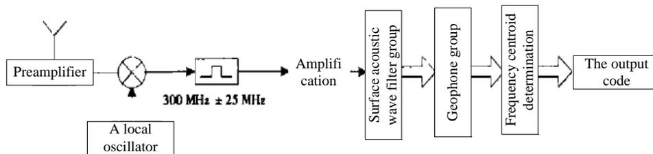
Figure 6 : Relation of IF channel receiver and the system
