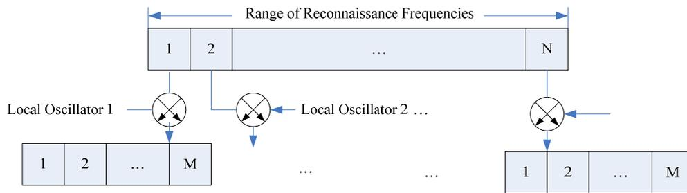
**Figure 1 : Schematic diagram of secondary pure channelized receiver**
