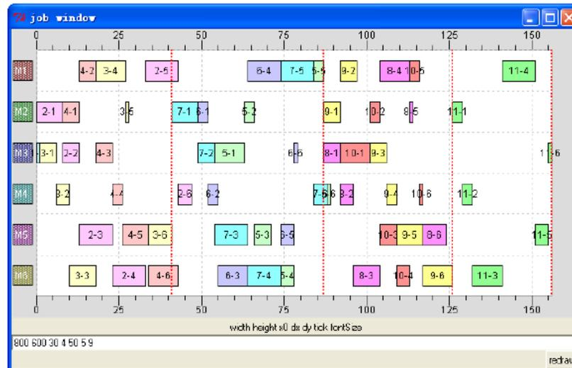
Figure 7 : Gantt chart of rolling-window-technology scheduling scheme
