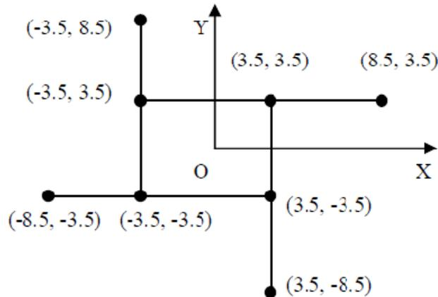
Figure 2: Typical 500kV tower grounding device
