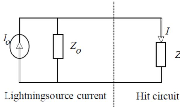
Figure 1: Equivalent circuit of lightning source current
