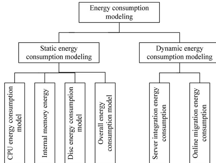
**Figure 2 : Classification of Energy Consumption Modeling Approaches of Virtualization Cloud Computing Platform**
