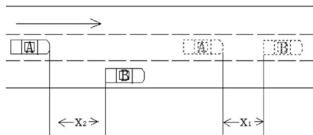
Figure 2 : Schematic plot of model 1 of changing lane to accelerate
