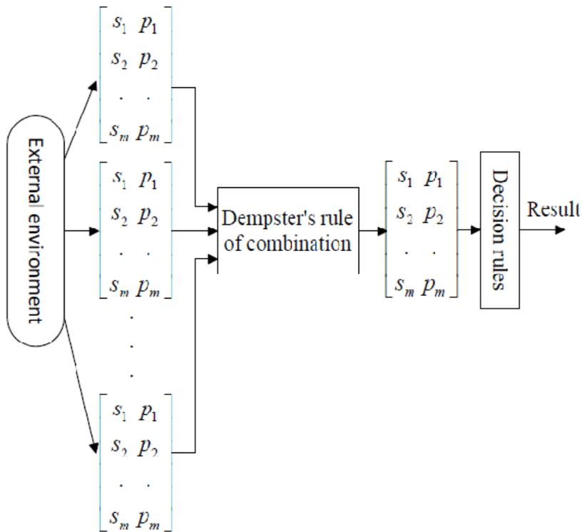
Figure 1: The theory of decision evidence of multiple sensor qualitative information fusion process
