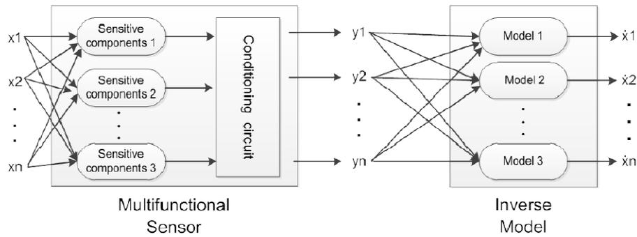
**Figure 5: Multifunctional sensor and its inverse model based signal reconstruction principle**
