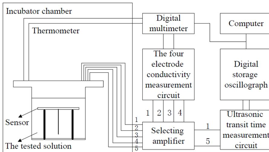
Figure 3: Multifunctional sensor signal reconstruction experiment data acquisition process
