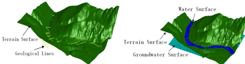
Figure 5 : Terrain model and geological line (1) Figure 6 : Groundwater and surface water level (1)
