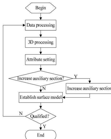
Figure 1 : Design of 3D modeling process
