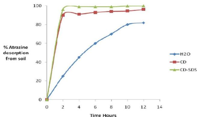
**Figure 5 :** Effect of  $\beta$ -cyclodextrin and SDS on the effectiveness of the atrazine extraction from the soil : The solvents used are respectively: H<sub>2</sub>O,  $\beta$ -CD [10mM], and [mixture of  $\beta$ -CD 10mM with SDS 0.1mM]
