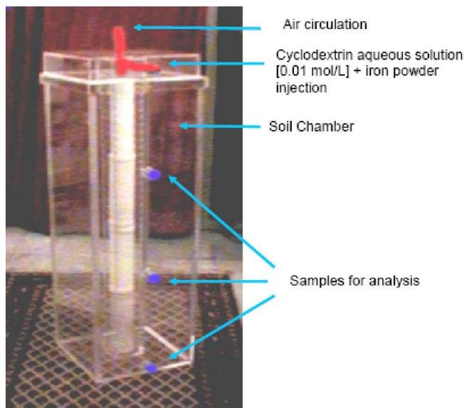
Figure 1 : Prototype soil column treatment using  $\beta$ -cyclodextrin, detergents and zero valent iron. Column external dimensions are 30 cm x 30 cm x 150 cm; and internal dimensions are 10 cm x 10 cm x 150 cm. This compartment is perforated from the bottom to the top. Sampling heights from the top of the column for analysis are: 5 cm, 55 cm, and 110 cm.
