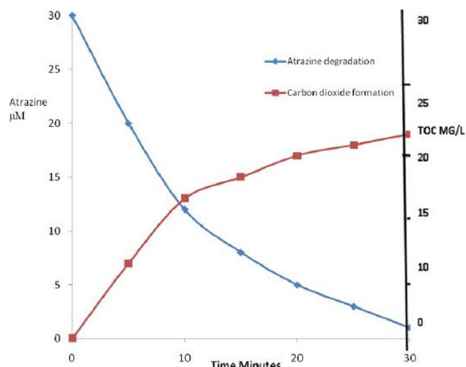
**Figure 8 :** Mineralization of atrazine and conversion into carbon dioxide as shown in the Figure . Blue is the degradation of atrazine. Red is the formation of carbon dioxide
