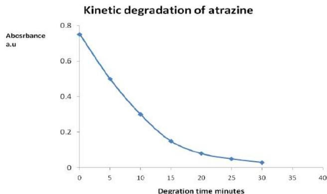
**Figure 7 :** Kinetic of atrazine degradation with the time of reaction- (minutes)
