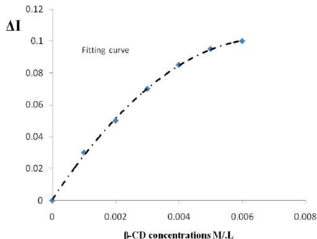
Figure 4 : Fitting curve of the guest-induced absorbance intensity ( $\Delta I$ ) vs. the initial concentration of the host  $\beta\text{-CD}$  ( $H_0$ ). Where  $\Delta I = (A-A_0)$ , and is equal to  $I_{\max} = (A_g - A_0)$  when every host exists as the inclusion complex
