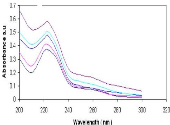
**Figure 2 :** UV/VIS absorption spectra of atrazine at  $9.26 \times 10^{-6}$  M in varying concentrations of  $\beta$ -CD solutions ( $1 \times 10^{-3}$  -  $9 \times 10^{-3}$  M). The higher concentrations of  $\beta$ -CD, corresponding to the higher absorbance.
