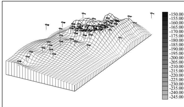
**Fig. 2: Three-dimensional model of confining reservoir bed**
