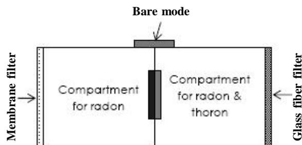
Figure 1: Entrenched outlook of Twin cup dosimeter
