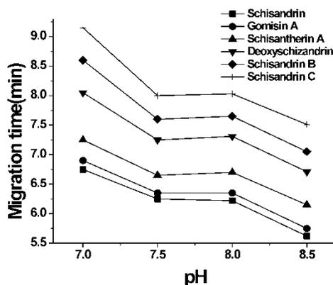
**Figure 2 :** Effect of varying the pH value of the buffer on mobilities of main lignans. Buffer: 30mM SDS and 35% v/v acetonitrile in 10mM phosphate. Applied voltage was 25 kV. Column temperature: 25.0 °C. Detection: 214 nm.
