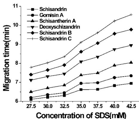
**Figure 3 :** Effect of varying the concentration of SDS on mobilities of main lignans. Buffer: 35% v/v acetonitrile and varying amount of SDS in 10mM phosphate(pH 8.0). Applied voltage was 25 kV. Column temperature: 25.0 °C. Detection: 214 nm.
