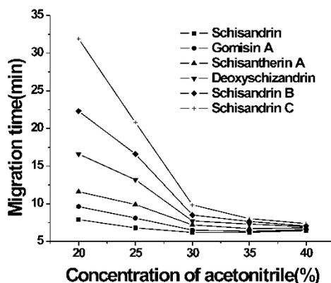
**Figure 1 :** Effect of varying the concentration of acetonitrile on mobilities of main lignans. Buffer: 30mM SDS and varying amount of acetonitrile in 10mM phosphate(pH 7.5). Applied voltage was 25 kV. Column temperature: 25.0 °C. Detection: 214 nm.
