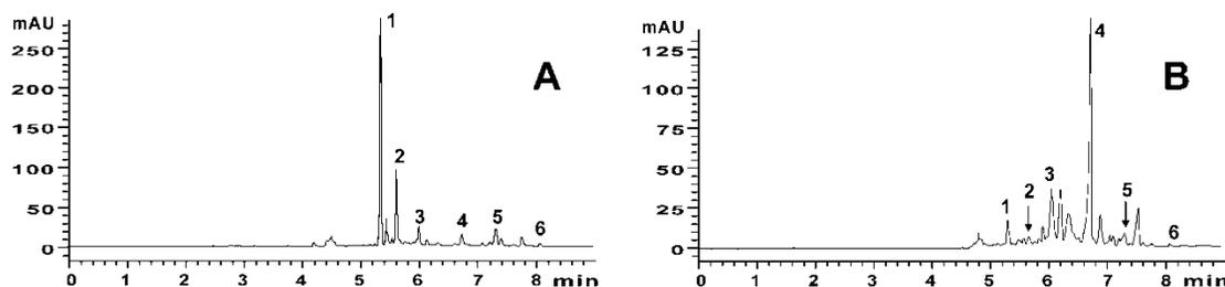
Figure 4 : Electropherograms of (A) *Schisandra chinensis* and (B) *Schisandra sphenanthera* Peak identification: 1, Schisandrin; 2, Gomisin A; 3, Schisantherin A; 4, Deoxyschizandrin; 5, Schisandrin B; 6, Schisandrin C. MEKC conditions: background electrolyte, 37.5mM SDS and 35% v/v acetonitrile in 10mM phosphate buffer (pH 8.0). Applied voltage was 28 kV. Column temperature: 25.0 °C. Detection: 214 nm.
