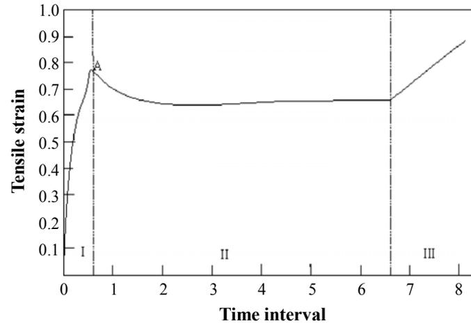
**Fig. 3: Curve of the load change on press-stem during the extrusion of section of the same type. Detail No. 2**
