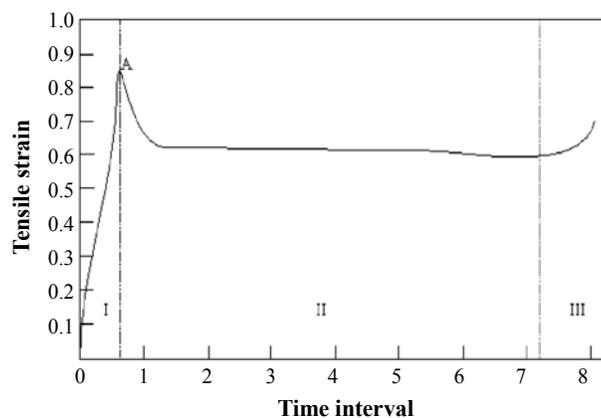
**Fig. 2: Curve of the load change on press-stem during the extrusion of section of the same type. Detail No. 1**
