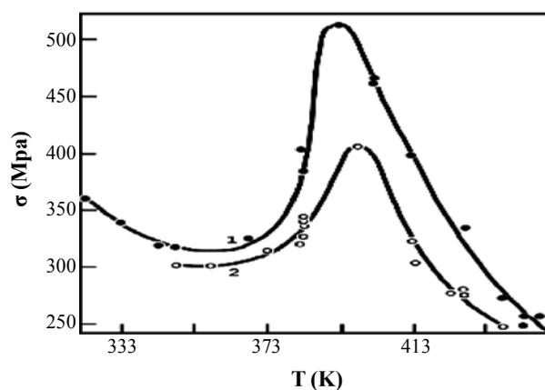
**Fig. 6: Temperature dependence of the yield strength of aluminum alloy D16**
