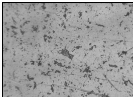
**Fig. 5: Surface of sample with small slag inclusions. Increase by x 100**
