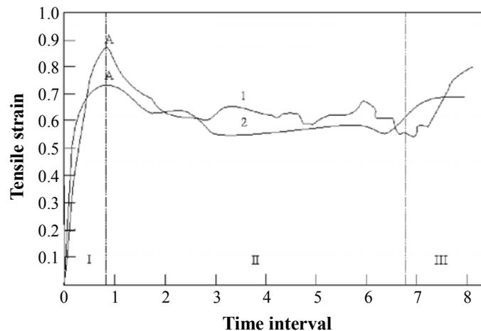
**Fig. 4: Curve of the load change on press-stem during the extrusion of section of the same type. Detail No.3 and No. 4**
