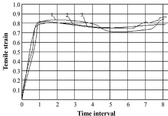
**Fig. 8: Curve of the load change on press-stem during the extrusion of section of the same type. Detail No. 1, 2, 3. Section No. 2**
