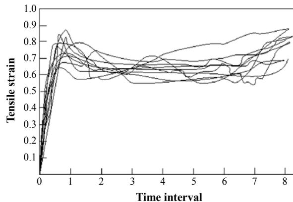
**Fig. 1: Loads change curves on press-stem during the extrusion of section of the same type**
