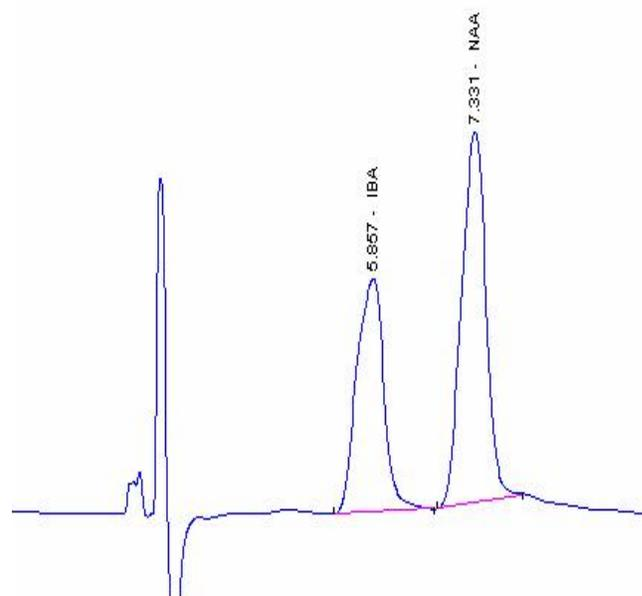
Figure 1 : Chromatogram of IBA and alpha-NAA when 65/35 v/v(0.1% pH 3.3) methanol : milli Q (formic acid buffer) was used as a mobile phase (flow rate 0.7 mL min<sup>-1</sup>)
