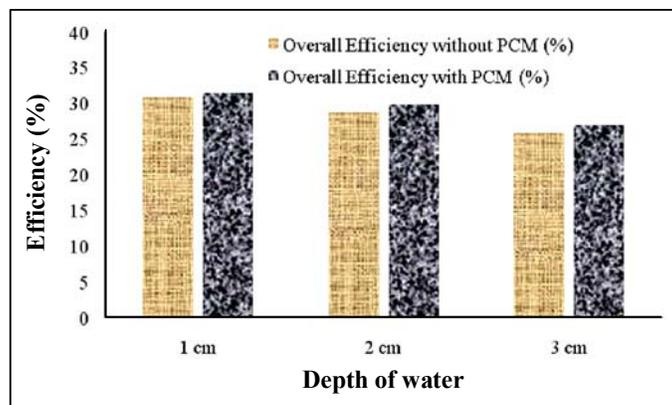
**Fig. 10: Variation of depth of water on efficiency**
