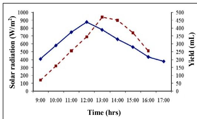
**Fig. 11: Radiation intensity and yield on 10 mm depth of water without PCM**
