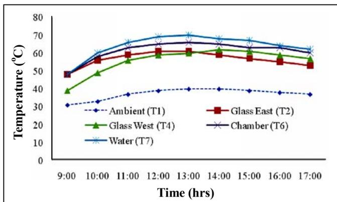
Fig. 2: Variation of temperature for 10 mm depth of water without PCM
