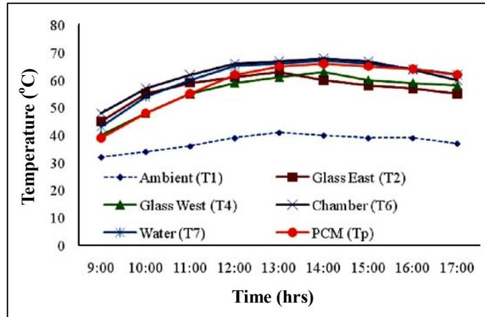
Fig. 5: Variation of temperature for 10mm depth of water with PCM
