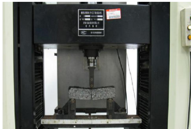
Figure 2 : Three-point bending fracture test setup
