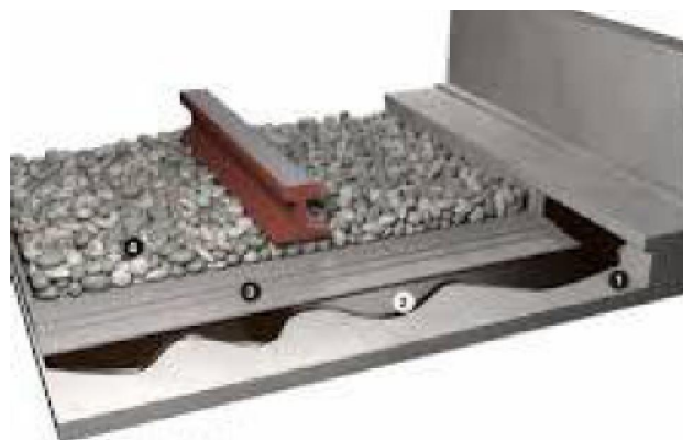
Figure 1 : The typical structure of the bridge deck system; 1. Substrate reinforced concrete 2. Waterproof coating 3. MAEC protective 4. Ballast
