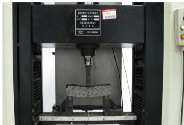
Figure 2 : Three-point bending fracture test setup
