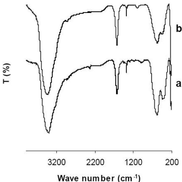
**Figure 2 :** FTIR spectra of a)  $\text{Fe}_3\text{O}_4/\text{P}(\text{S-NIPAM})$  composite seed, and b)  $\text{Fe}_3\text{O}_4/\text{P}(\text{S-NIPAM})/\text{P}(\text{NIPAM-MAA-MBAAm})$  composite polymer particles recorded in KBr pellets
