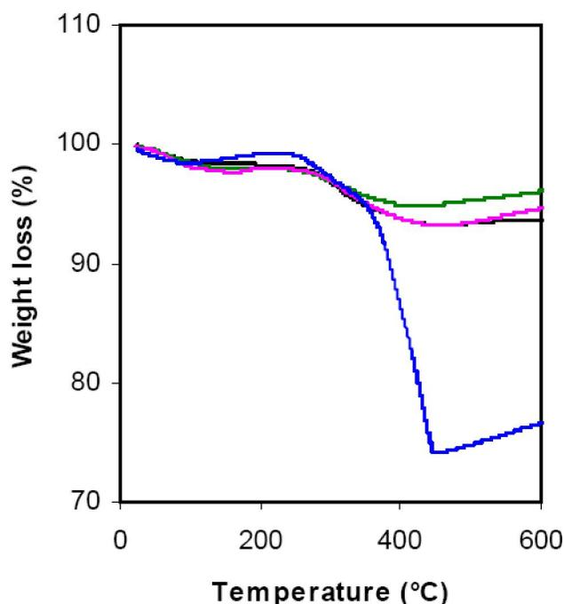
**Figure 3 :** TGA thermograms of  $\text{Fe}_3\text{O}_4$  (black line), functionalized  $\text{Fe}_3\text{O}_4$  (green line),  $\text{Fe}_3\text{O}_4/\text{P}(\text{S-NIPAM})$  (pink line) composite seed, and  $\text{Fe}_3\text{O}_4/\text{P}(\text{S-NIPAM})/\text{P}(\text{NIPAM-MAA-MBAAm})$  (blue line) composite polymer particles
