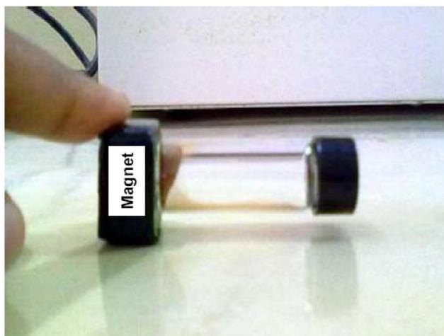
**Figure 5 :**  $\text{Fe}_3\text{O}_4/\text{P}(\text{S-NIPAM})/\text{P}(\text{NIPAM-MAA-MBAAm})$  composite particles being attracted by a magnet
