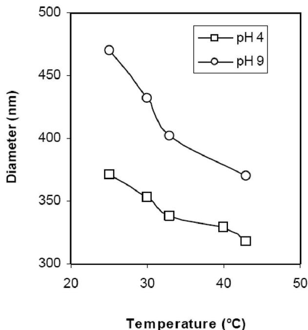
**Figure 4 :** Variation of average hydrodynamic diameter of washed  $\text{Fe}_3\text{O}_4/\text{P}(\text{S-NIPAM})/\text{P}(\text{NIPAM-MAA-MBAAm})$  composite polymer particles at pH 4 and 9 against temperature
