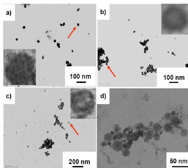
Figure 1 : TEM photographs of a)  $\text{Fe}_3\text{O}_4$ , b) functionalized  $\text{Fe}_3\text{O}_4$ , c)  $\text{Fe}_3\text{O}_4/\text{P}(\text{S-NIPAM})$  composite seed, and d)  $\text{Fe}_3\text{O}_4/\text{P}(\text{S-NIPAM})/\text{P}(\text{NIPAM-MAA-MBAAm})$  composite polymer particles
