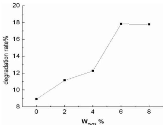
Figure 1 : Degradation rate of Rhodamine B solution containing different concentration TiO<sub>2</sub> transparent emulsion
