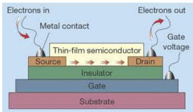
Figure 2 : Thin film transistor
