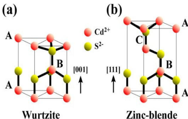
Figure 1 : Crystal structure of CdS in (a) Wurtzite and (b) Zinc-blende symmetries
