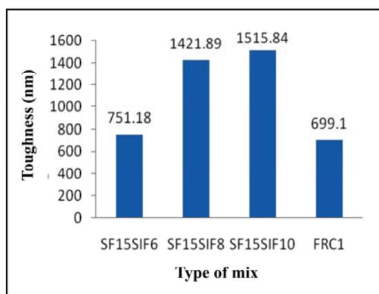
**Fig. 9(a): Type of mix vs Toughness**
