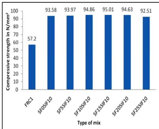
Fig. 3(a): Type of mix vs Compressive strength
