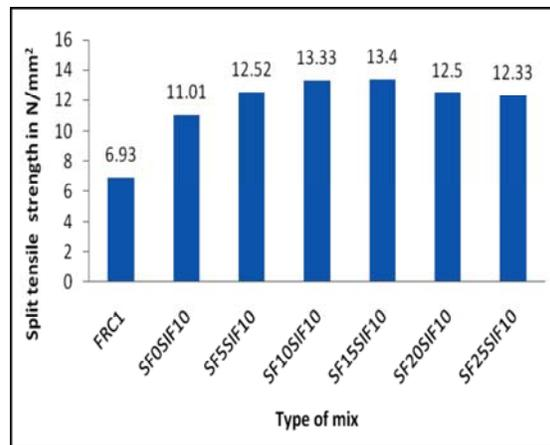
Fig. 3(b): Type of mix vs Split tensile strength
