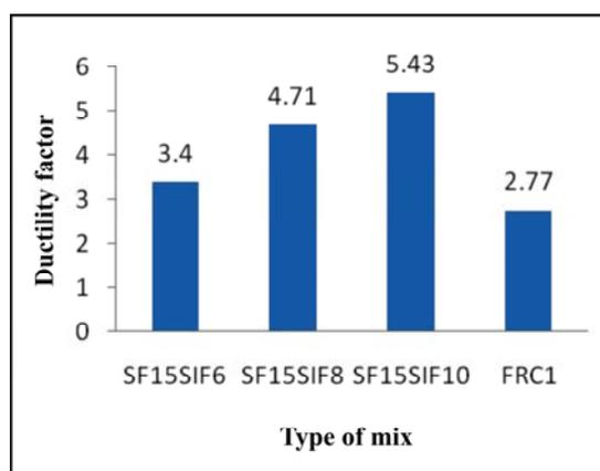
**Fig. 9(b): Type of mix vs Ductility factor**
