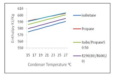
Fig. 4: Variation condenser temperature with Enthalpy
