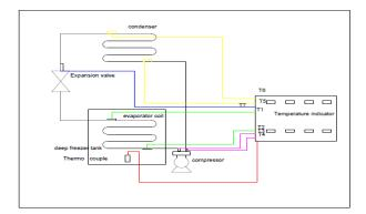
Fig. 1: Measuring locations of the test deep freezer setup
