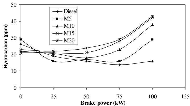
**Fig. 7: Hydrocarbon emission Vs brake power**
