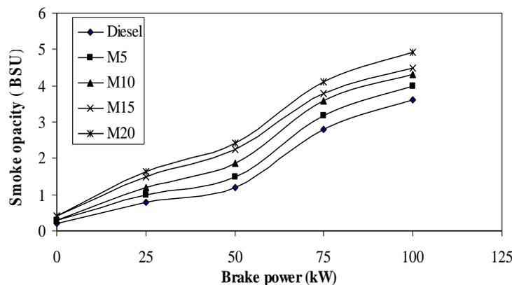
**Fig. 9: Smoke opacity Vs brake power**
