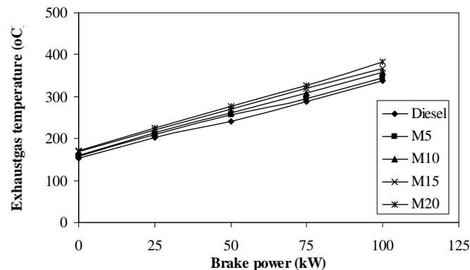
**Fig. 5: Exhaustgas temperature Vs brake power**
