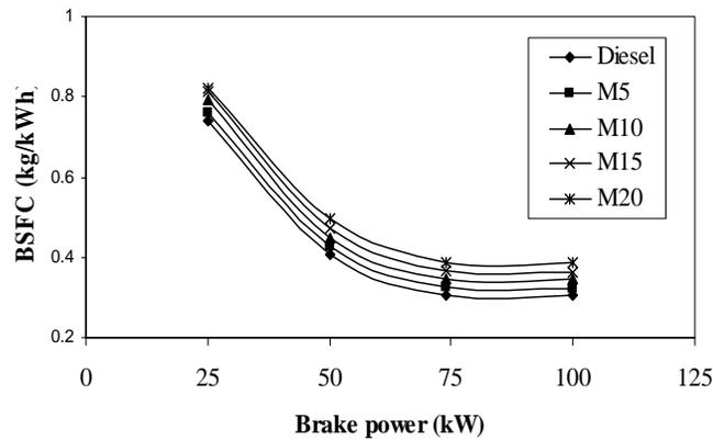
**Fig. 4: Brake specific fuel consumption Vs Brake power**
